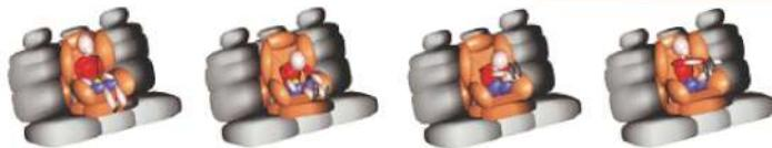
Using dummies specifically designed for this kind of impact (BIORID II) we analyse the most up-to-date systems to avoid injuries related to whiplash in rear impacts.
